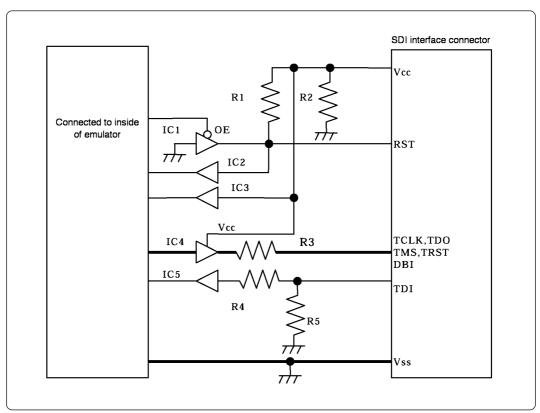
Figure 3.5 Circuit diagram of the emulator side of the SDI interface
